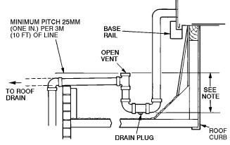
NOTE: Trap should be deep enough to offset maximum unit static difference. A 100 mm (4 in.) trap is recommended.
